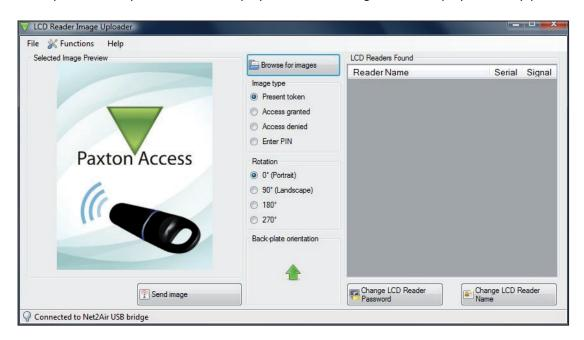
Run the LCD reader image uploader and it will detect the USB Net2Air device connected to the PC. The PC will then detect and display any LCD units that are in range of the USB device.
